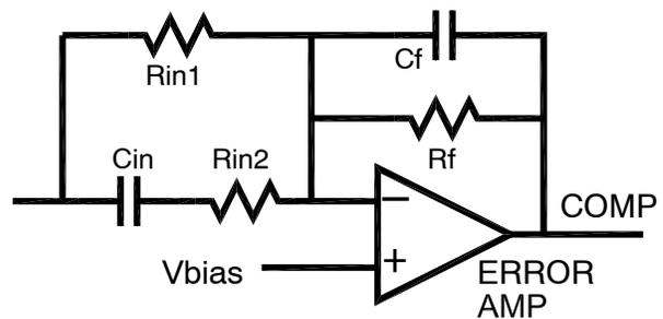
**Figure 5. NCP81142 Modified Type 3 External Compensation**
